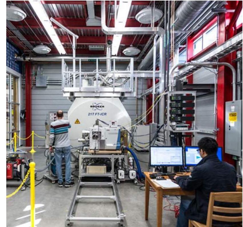
21 T FT-ICR MS system at National High Magnetic Field Laboratory – MagLab (Florida, USA)
