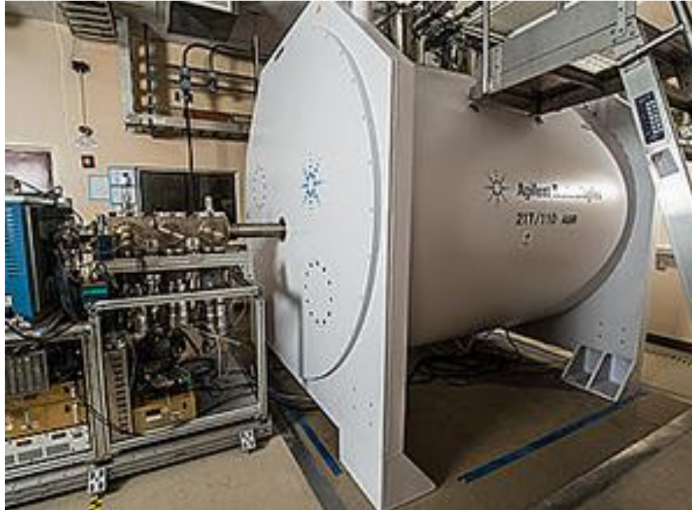
21 T FT-ICR MS system at Pacific Northwest National Laboratory – PNNL (Washington, USA)
